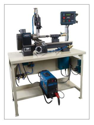
the setting of rotational speed and the delays for the starting and stopping of travel. The control indicates speed before and during welding.
